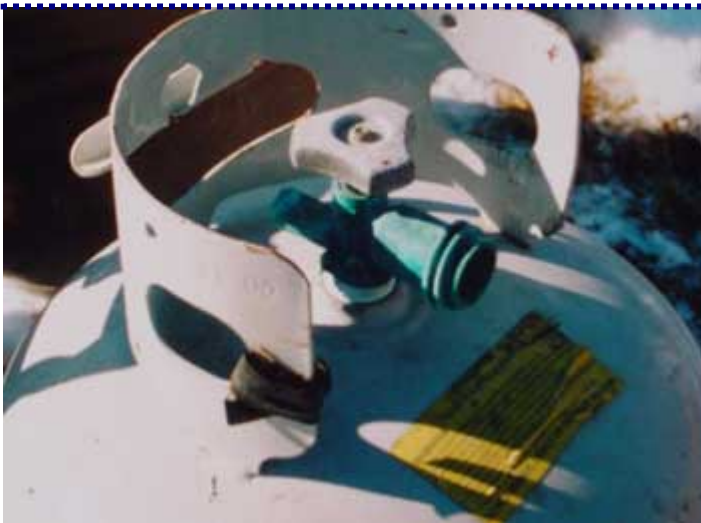
Photo showing blue valve caused by storage of ammonia
