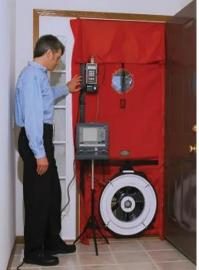
Air Changes per Hour at 50 Pascals (ACH50) – The number of times in an hour that the total air volume of a home is exchanged for outside air with the house depressurized or pressurized by a blower door to 50 Pascals with reference to the outside. Pascals – A measurement of air pressure. One inch of water column is equal to 249 Pascals.
