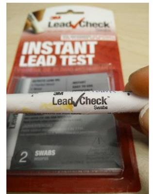
**Figure 1:** Contractors use kits like this 3M™ LeadCheck™ to test for the presence of lead after doing renovations and remodels in pre-1978 housing.
