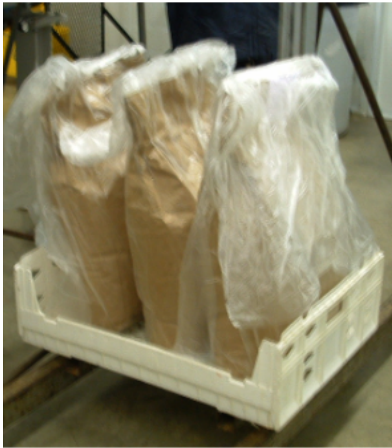
Figure 1. Kraft 22.7 kg bags of pellets in polypropylene overwrap bags.
