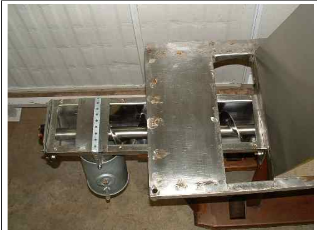
Figure 4. Five inch auger connected directly to the mixer.
