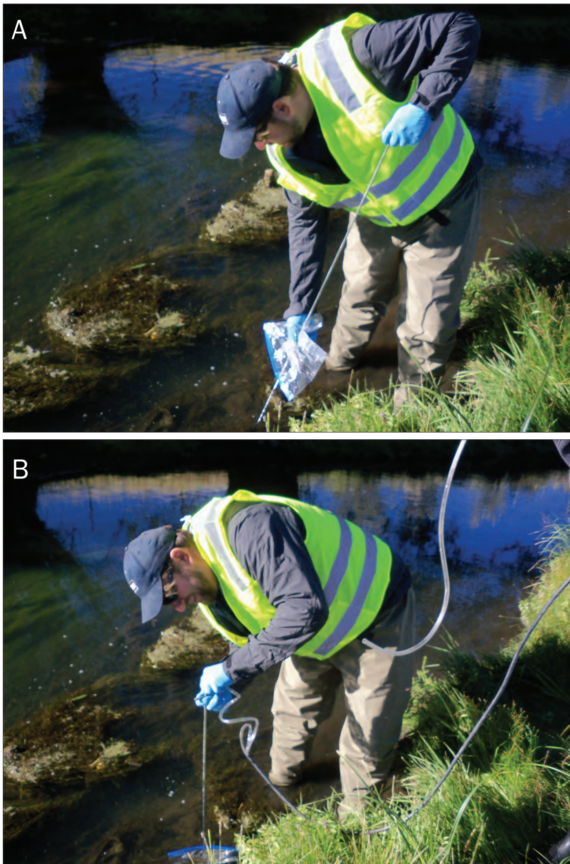
Figure 5. Synoptic drive-point samples of streambank groundwater were collected at five locations during the tracer test. (A) CDM-Smith representative pushing sampler into streambed sediment. (B) CDM-Smith representative attaching tubing to sampler head. Samples were purged via peristaltic pump into bulk 1-gal containers.
