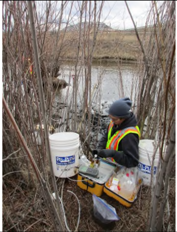
PHOTOGRAPH 10 Collecting surface water and pore water samples at sample point BTC-05N.
