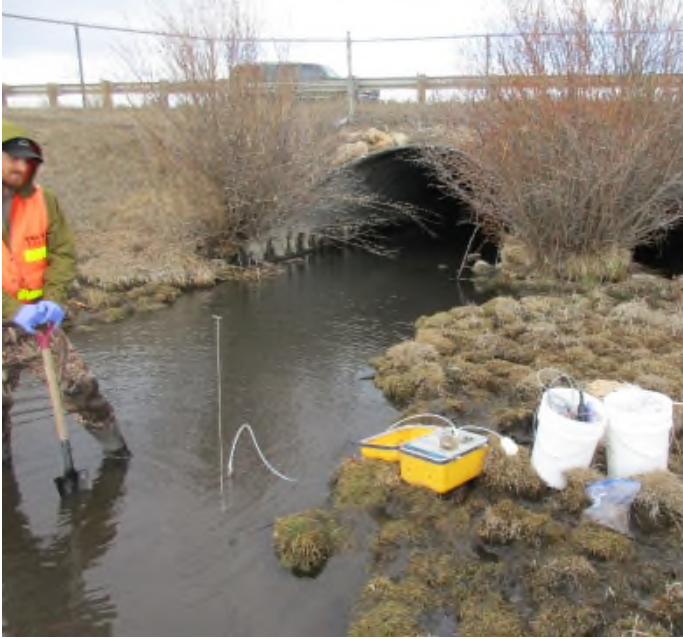
PHOTOGRAPH 9 Collecting a pore water sample near confluence of Sand Creek and Blacktail Creek, at sample point SC-01.
