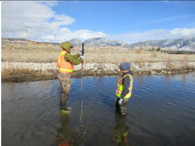
PHOTOGRAPH 7 Collecting a streambed sediment sample at BTC-01 using the AMS™ slide hammer sediment sampling apparatus.
