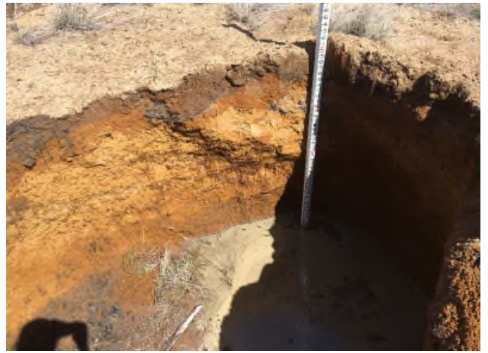
PHOTOGRAPH 6 Test pit BTC-TP-11, with orange sand and debris to 4 ft bgs, with groundwater at 4 ft bgs.
