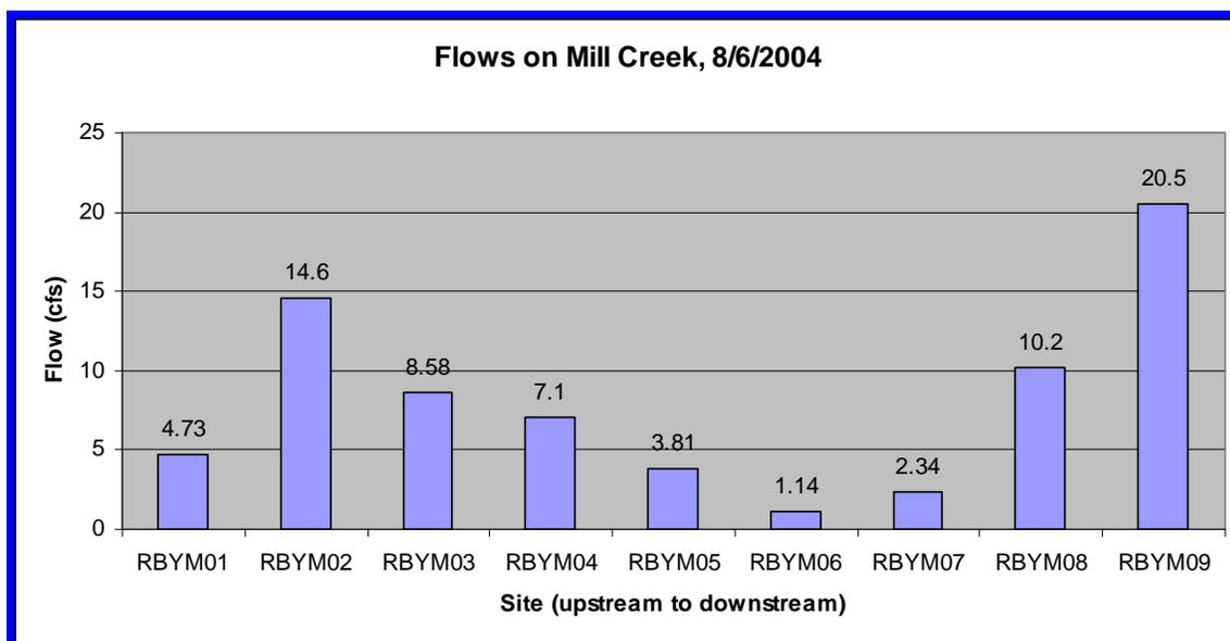
**Figure 1. Trends in Streamflow on Mill Creek on August 6, 2004. Sites are Listed Left to Right from Upstream to Downstream.**
