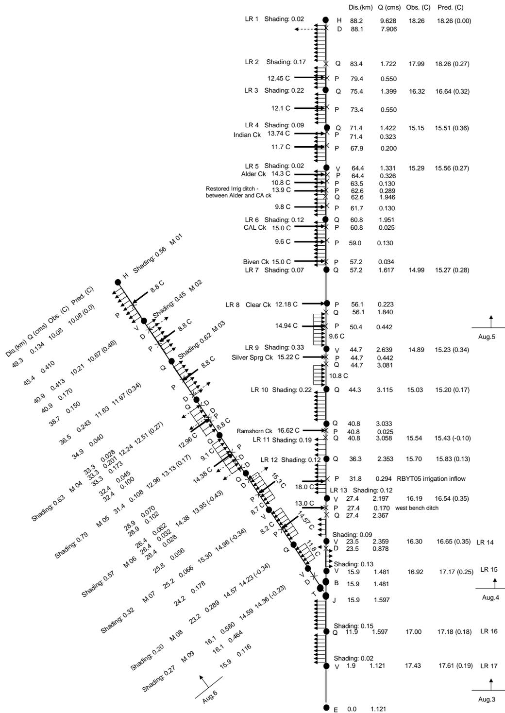
**Figure A1. Schematics of the Ruby River systems as represented in SNTemp\***
