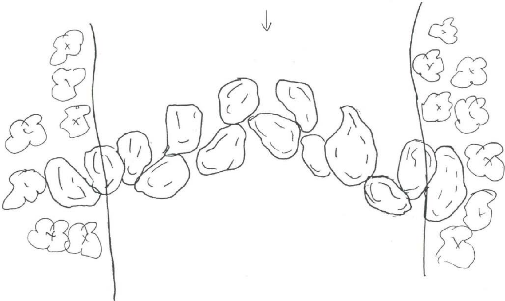
Figure 5e. Plan view of vortex rock weir to be used for grade control, reduction of bank erosion and improvement of fish habitat in alterations of F4 channel types to B4 channel types.
