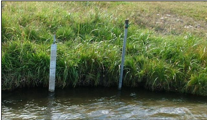
Figure 2: Reference Staff gage and stilling well deployed in field (Big Pipestone Creek, 2010)
