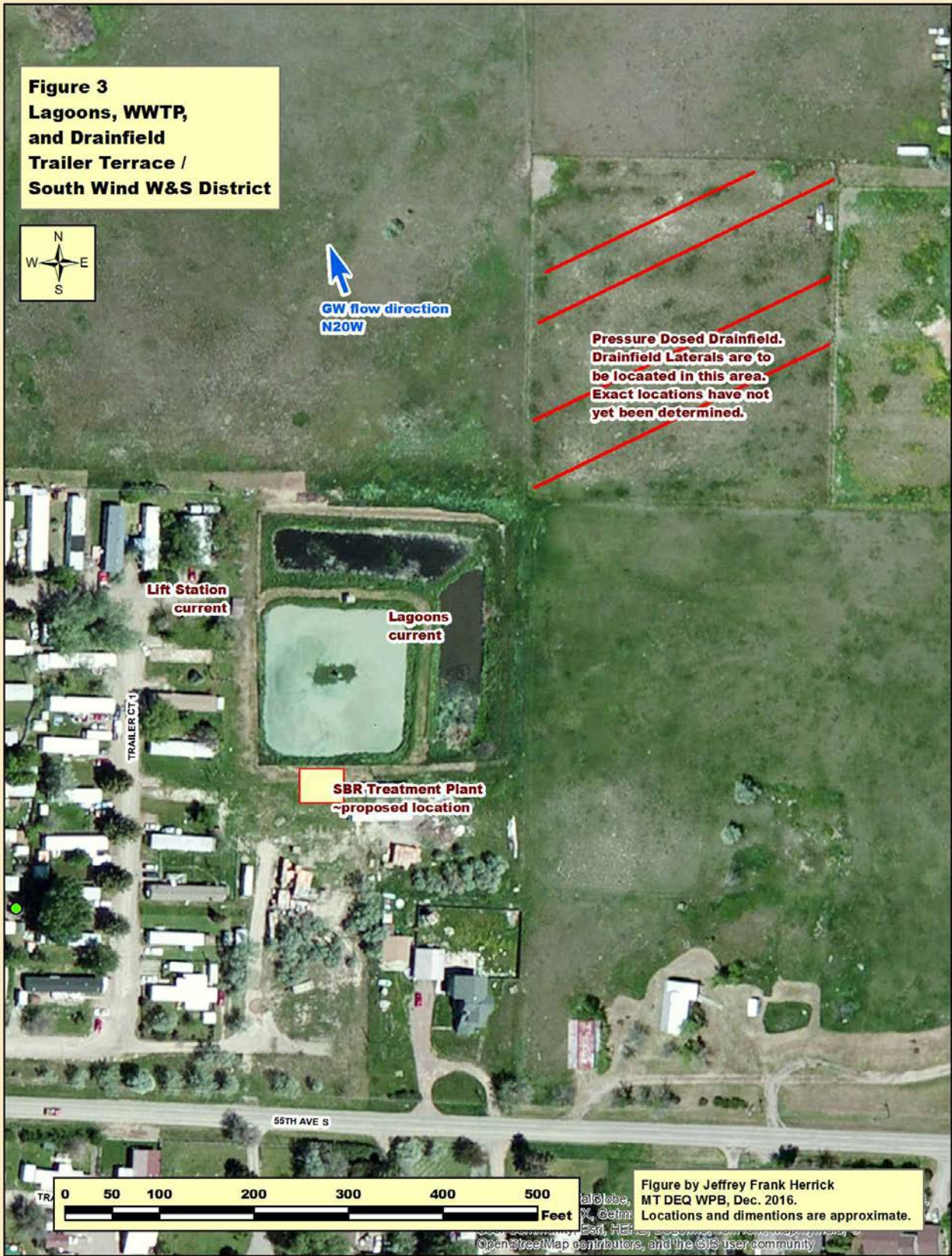
FIGURE 3 – Lagoons, Plant, & Drainfield
