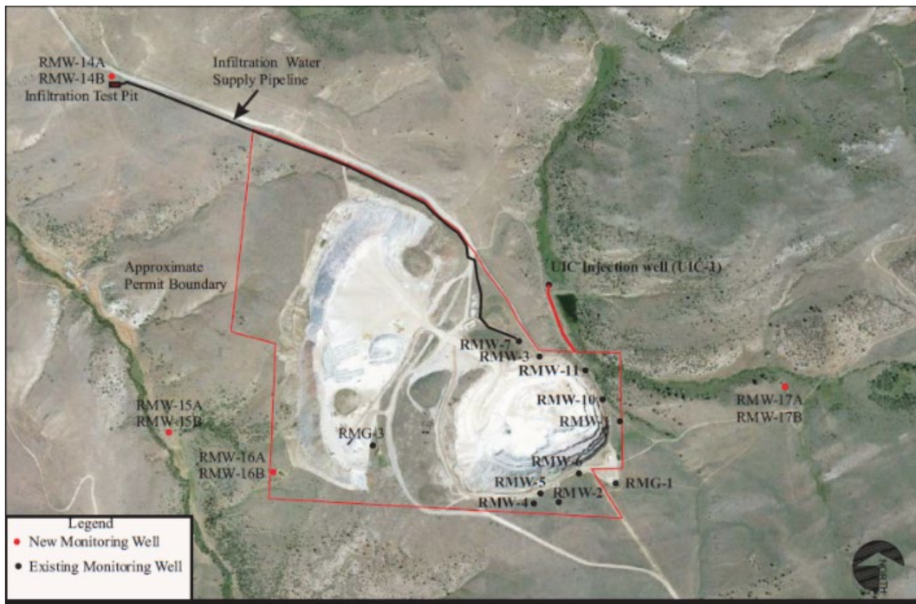
Figure 3.4-3 Proposed and Existing Ground Water Monitoring Wells (Hydrometrics, Inc. 2019c)
