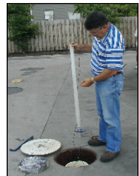
Bailing A Groundwater Monitoring Well
