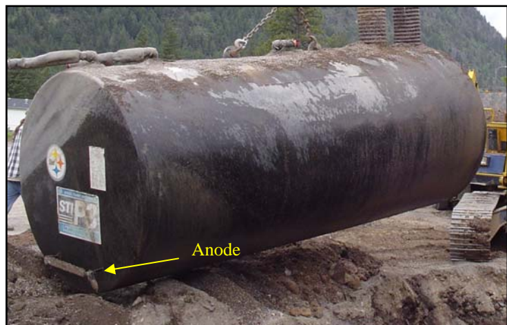
Tank with Galvanic cathodic protection (Notice the sacrificial anode on the end)
