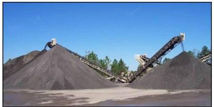
RAP processing and fine and coarse aggregate stockpiles at an asphalt concrete production plant - photo courtesy US DOT website
