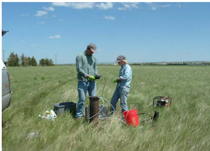
SRS staff using DEQ's new QED MicroPurge Flow Cell and Portable Pump
