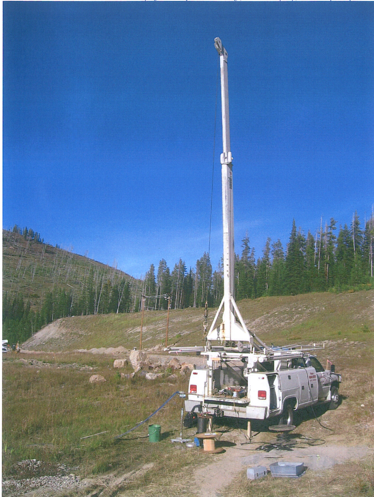
INSERT DAILY PHOTO WITH CAPTION: Pumping of C1-2 by O'Keefe drilling (Chamberlain pump). Note new power poles in background.
