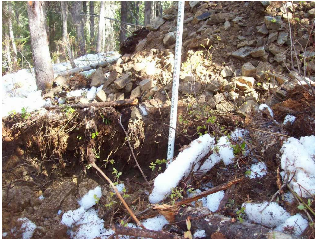
Test pit excavation at Road Bench Site #2
