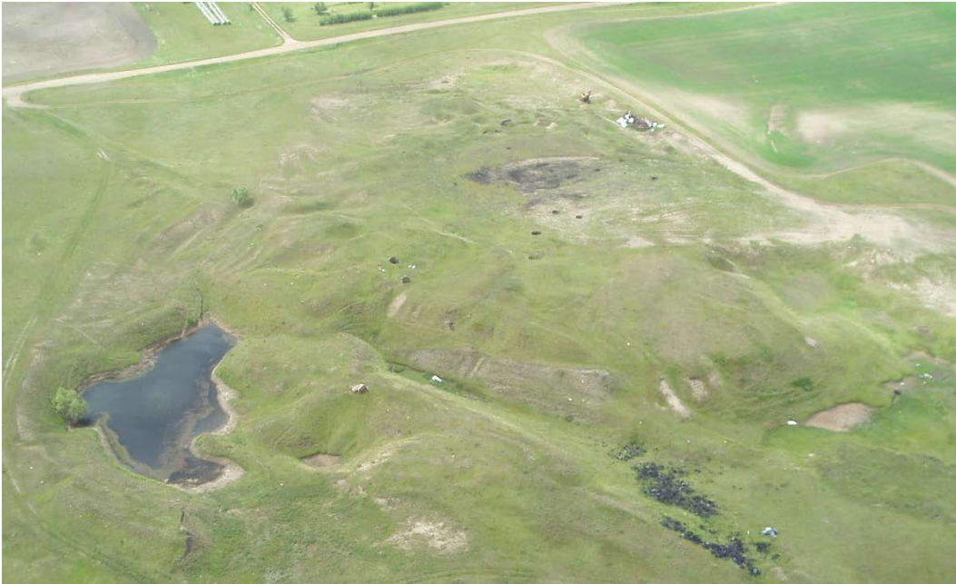
Figure 6. Subsidence at the Wheeler Langerquist Coal Mine.
