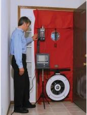
Air Changes per Hour at 50 Pascals (ACH50) – The number of times in an hour that the total air volume of a home is exchanged for outside air with the house depressurized or pressurized by a blower door to 50 Pascals with reference to the outside.
