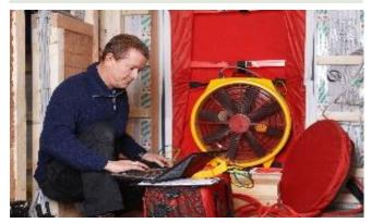
The basic blower door test on a single family home measures only the leakage through the exterior envelope, which is all leakage to the outside. This leakage includes leakage through ducts located outside the thermal envelope. In multifamily buildings a simple one fan blower door test on a single unit will measure leakage to the outside and leakage to the adjacent spaces.
