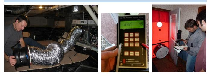
A duct tightness test involves the use of a duct tightness fan (shown above at the left), a digital manometer (center), and in the case of a duct leakage to the outside test, a blower door fan (right).
