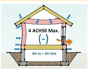
possibility that asbestos or other unwanted dust or particles may be present in the building cavities. A pressurization blower door test usually takes longer to perform since the exhaust backdraft dampers must be sealed before testing occurs.
