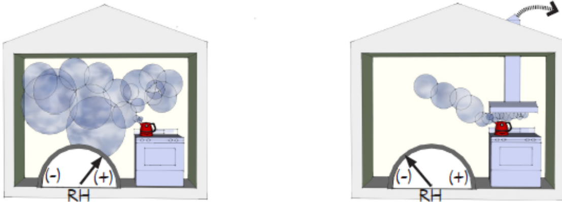
Figure 7 EXHAUST VENTILATION CAN REDUCE HUMIDITY LEVELS
