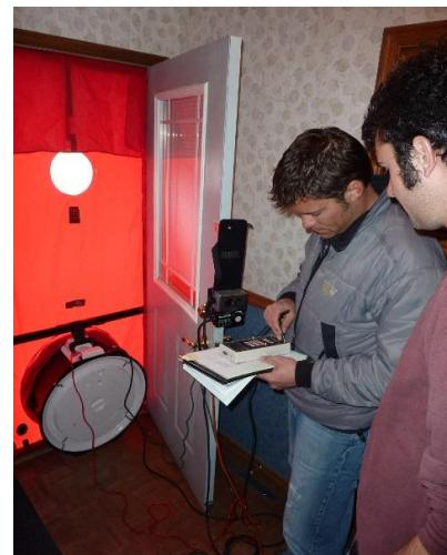
A duct tightness test involves the use of a duct tightness fan (shown above at the left), a digital manometer (center), and in the case of a duct leakage to the outside test, a blower door fan (right).
