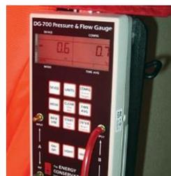
**Air Changes per Hour at 50 Pascals (ACH50)** – The number of times in an hour that the total air volume of a home is exchanged for outside air with the house depressurized or pressurized by a blower door to 50 Pascals with reference to the outside.
