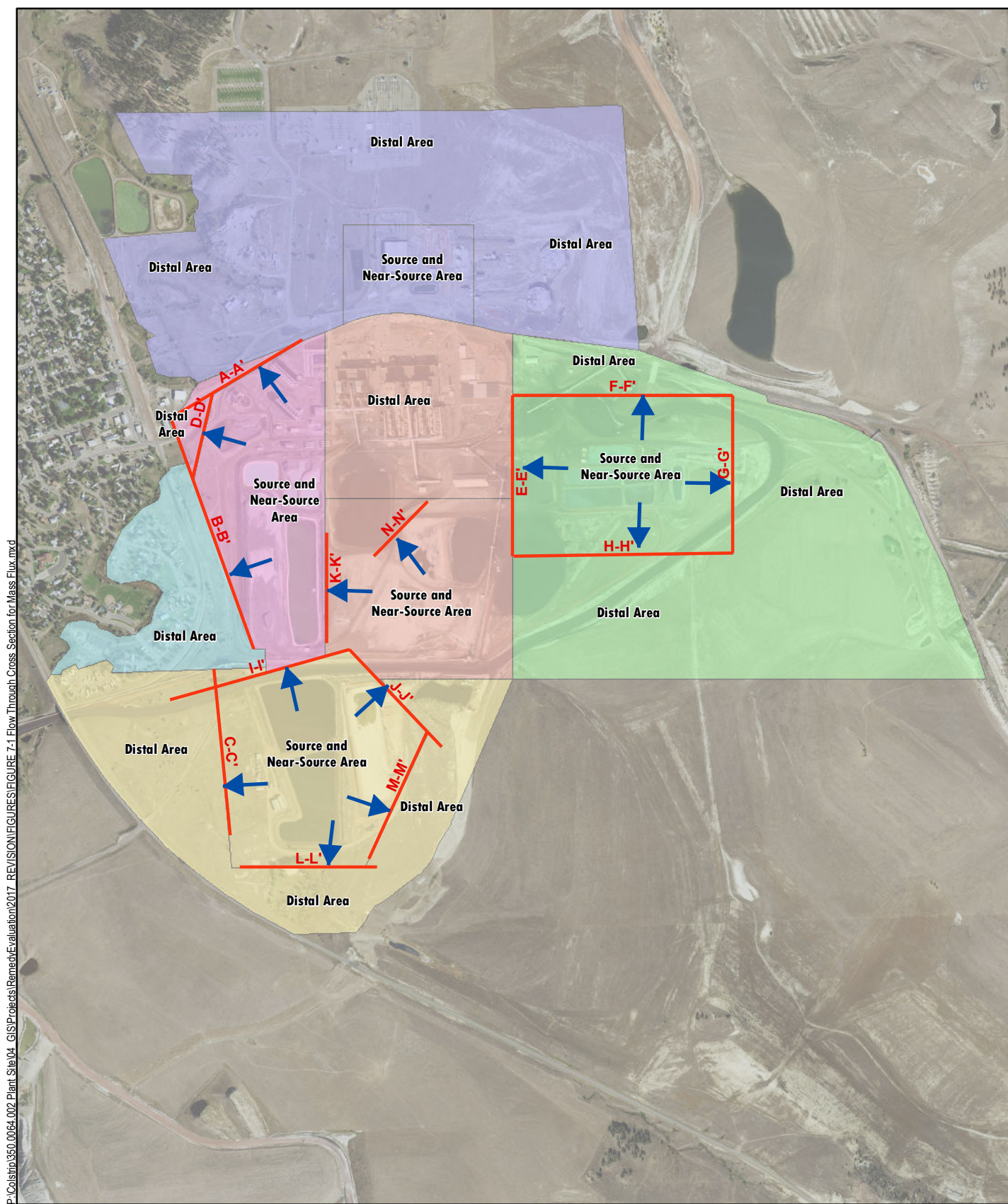
Direction of Groundwater Flow through Transects for Mass Flux Calculations Plant Site Area Remedy Evaluation CSES-Colstrip, Montana FIGURE 7-1
