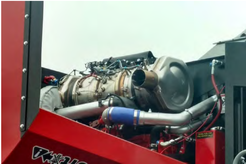
Tier 4 exhaust on a Log Loader. This is exhaust, but looks like a jet engine.
