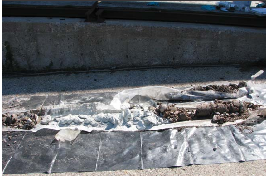
Soil cuttings from boring BB003 (Glue/resin wastewater tank).
